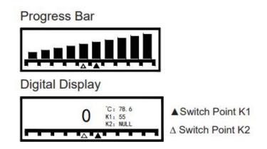
When Switch Point Sign light is flashing, it indicates that the velocity exceeds the switch action velocity
